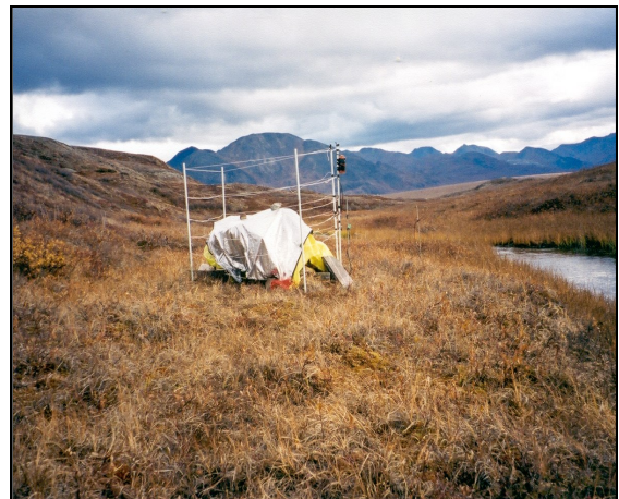
Portable electric fence around game meat in Alaska. Photo courtesy of Jamie Jonkel, Montana Fish, Wildlife & Parks.
